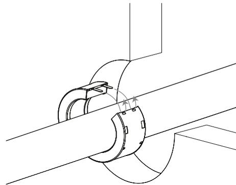
2. Remove the label. Open the fire collar and place it around the pipe.
