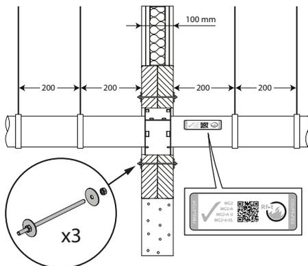
7. Put 3 threaded rods through the stone wool boards and fix with M6, washers and bolts. Apply the label nearby the collar.
