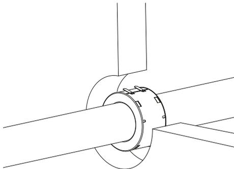
3. Slide the collar into the opening of the wall, in the middle of the wall thickness.
