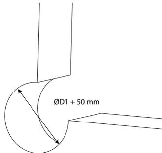
1. Provide an installation opening of  $\text{ØD1} + 50 \text{ mm}$ .
