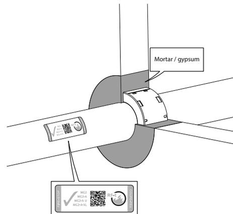
4. Seal with standard mortar (floor) or plaster (vertical wall).
