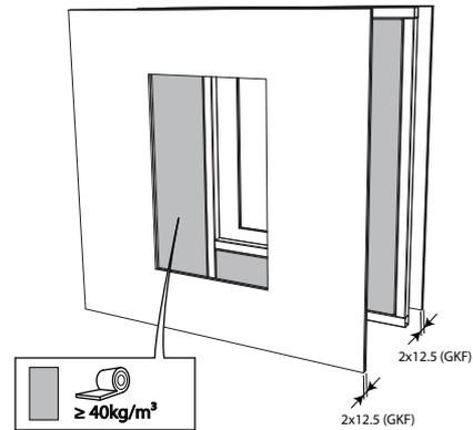
2. Fix two gypsum plasterboards type F of 12,5 mm thickness to each side of the metal studs and insulate the wall with 40 mm mineral wool, 40 kg/m<sup>3</sup>.
