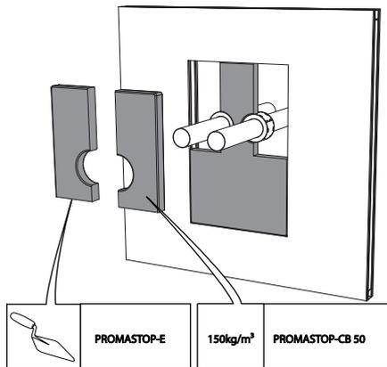
5. Fix a stone wool board of min. 50 mm thickness with fire resistant coating on one side (type PROMASTOP-CB 50) around the fire collars. Use a saw or knife to dimension the stone wool boards. Apply endothermic coating (type PROMASTOP-E) on the lateral sides, as well as on the joints.
