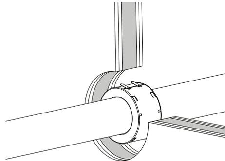
4. Slide the collar into the opening of the wall, in the middle of the wall thickness.
