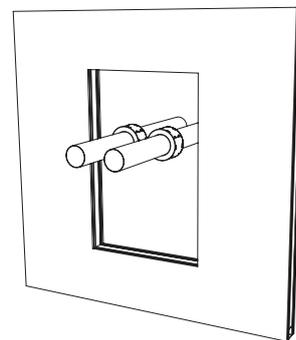
4. Place the built-in fire collars around the pipes by removing the label and fixing the collar by bending the fastening strips. Position the collars in the middle of the wall thickness.
