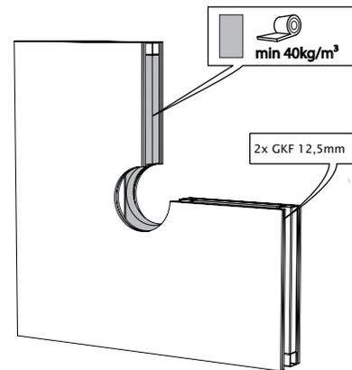
2. Insulate the wall and finish with two gypsum plasterboards type F.
