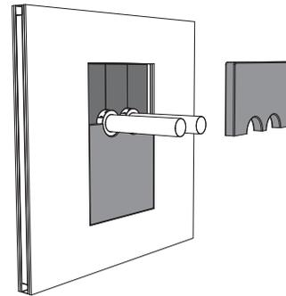
6. Put the second stone wool board of min. 50 mm thickness around the collars. Avoid the joints from coinciding. Apply endothermic coating (type PROMASTOP-E) on the lateral sides, as well as on the joints.
