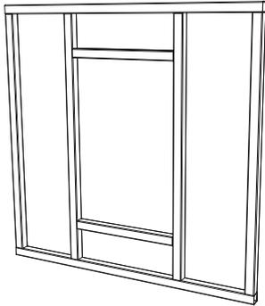
1. Provide an installation opening of maximally 1000 x 600 mm.
