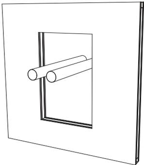
3. Place the plastic pipe(s). The distances between the pipes and the edges of the seal are min. 100 mm.
